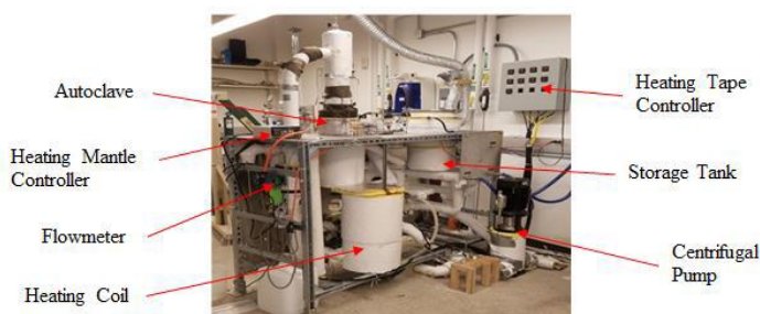
Fig.8 High-temperature water loop
